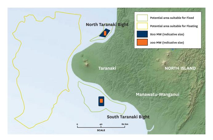
Initial analysis suggests the areas potentially suitable for offshore wind utilising fixed turbines in South and North Taranaki waters are 1,800 km² and 370 km² respectively (the areas in green in Figure 3). If fully developed these areas could deliver 12 GW and 2.4 GW respectively, and would double New Zealand's current electricity supply.
